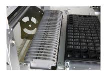
**Electronic feeders**, adopts feeding error corrections technique to help smooth the picking and reduce the deviation
