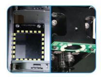
**Dual vision system**(up-looking and down-looking cameras), equip with high speed industry CCD cameras can help to identify and calibrate the four picking components at one time, highly improved accuracy of placement from 0201 to BGA
