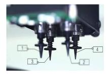
**Four high precision nozzles**, after calibration by vision software, it can reach to pick and place four components at one time with 360 degrees rotation at -180 to 180
